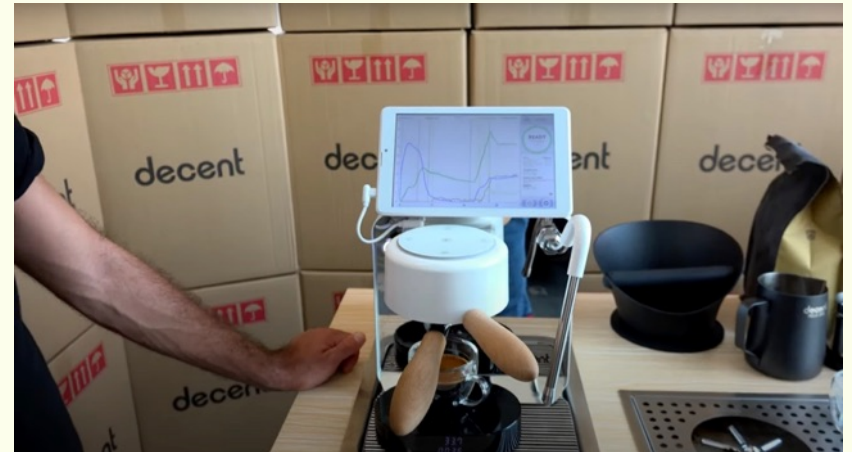
The portafilter and the group head handle, side by side
