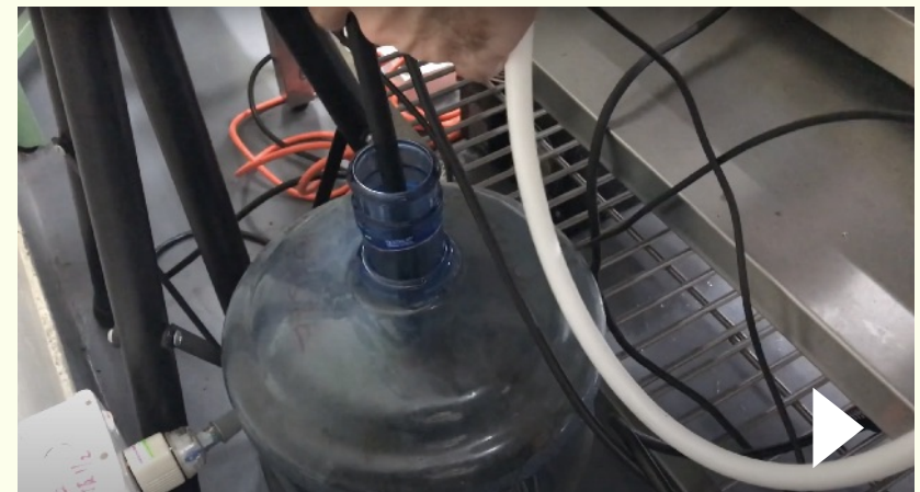
Waste water drains from the drip tray through a black tube to a bottle for disposal.
