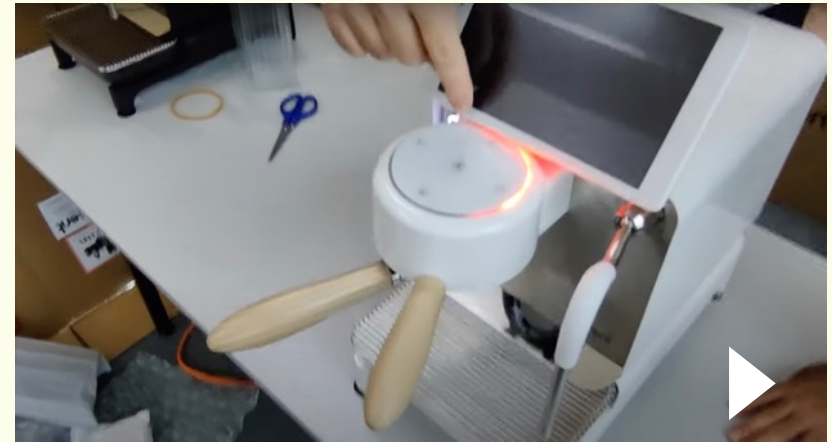
The Decent machine cycling through tests and warmup.
