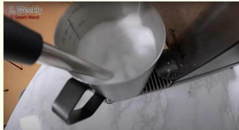
Frothing the steam wand in a solution of Rinza and water.
